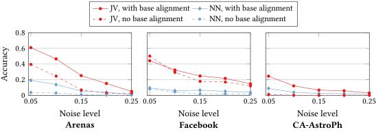
Fig. 10. Accuracy of nearest neighbor and JV matching algorithms with and without base alignment.
