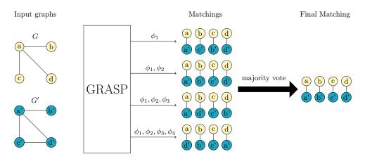
Fig. 3. An example of the voting heuristic in action; GRASP runs four times, adding one eigenvector in each iteration, from  $\phi_1$  to  $\phi_4$ . We omit eigenvectors  $\psi_1, \ldots, \psi_4$  for the sake of readability. Each set of eigenvectors returns a matching from nodes a, b, c, d to a', b', c', d'; on node a the match a-a' is selected by 3 out of 4 eigenvector sets and chosen as the output match.
